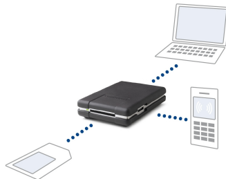
Figure 2.3: Monitoring of smart card communication using a COMPRION monitoring hardware. The traced data stream is passed to the monitoring application residing on a computer, where the parsing, monitoring and further analysis are performed.
