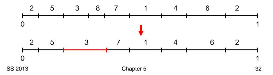
Consistent hashing works well for processes of uniform capacities.
