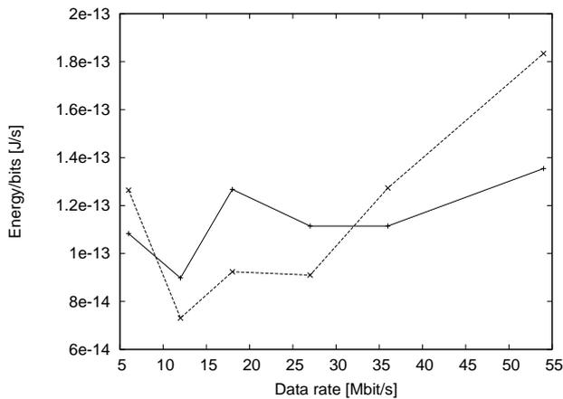
**FIGURE 10.** Received energy per goodput bit vs. data rate when comparing relaying with direct transmission
