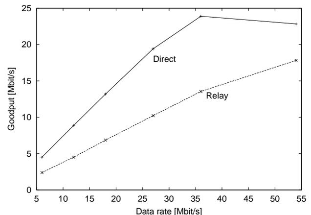
**FIGURE 9.** The resulting network capacity (throughput)
