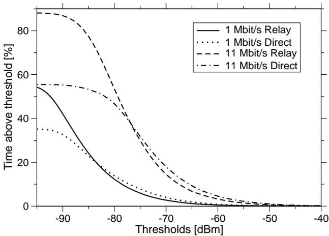
**FIGURE 7.** Comparison of distribution functions of relative share of time for which a given threshold value is exceeded, 1024 Byte packets, 25% load
