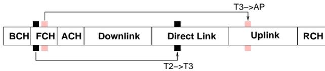
FIGURE 3. Relaying within the HIPERLAN/2 frame structure
