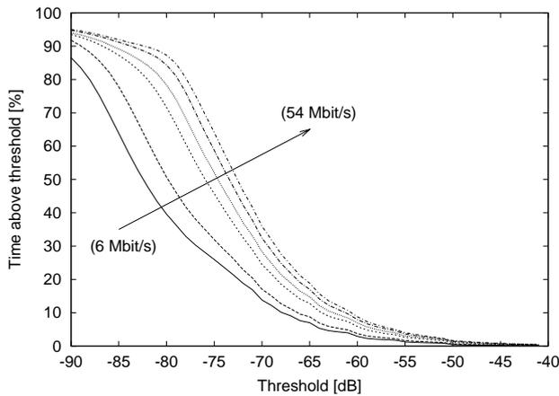
**FIGURE 11.** Percentage of time for which the received power exceeds a given threshold level; all data rates are shown; direct case
