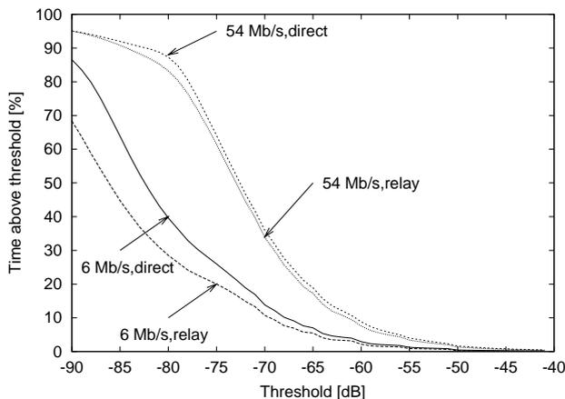
**FIGURE 12.** Percentage of time for which the received power exceeds a given threshold level; highest and the lowest data rate for the direct and the relay case are shown
