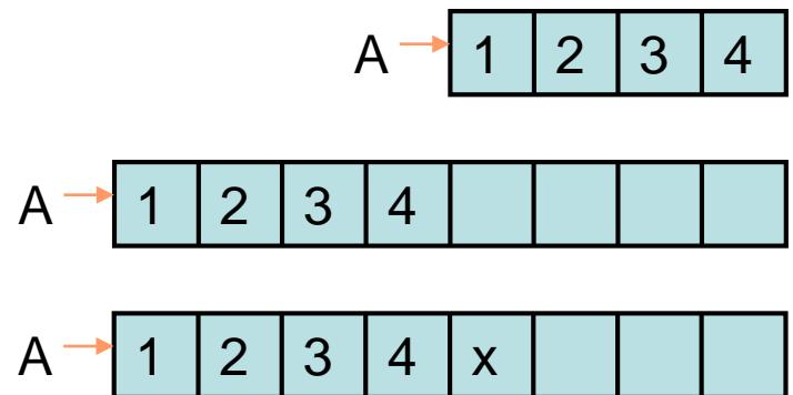
realloc(A,w): allocate array B of size  $w$ , copy contents of A to B, and return B
